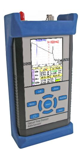
The NT2-210019 is a Tunable DWDM OTDR with 97.5 wavelengths from the C-Band spectrum. These 97.5 wavelengths are available in a single hand-held, tunable OTDR. The ODTR also operates as Tunable Light source with 6 dB power output range. Use the ODTR for commissioning and troubleshooting DWDM Metro Ethernet Networks.
