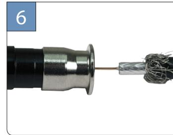
6 Insert the cable into the back of the connector and into the floating pin. Push the connector on while rotating until fully seated.
