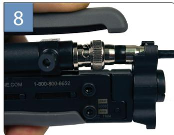
8 Using your VT-HE compression tool, make sure the rotating compression head is positioned for BNC as shown in the picture. Properly seat connector and compress fully.
