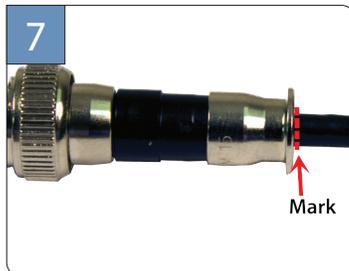
7 The cable mark from step 5 should line up with the back edge of the compression ring.
