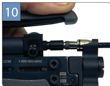
10 Using your VT-HE compression tool, make sure the rotating compression head is positioned for MCX as shown in the picture. Properly seat connector and compress fully.
