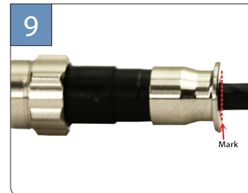
9 The cable mark from step 5 should line up with the back edge of the compression ring.
