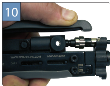
10 Using your VT-HE compression tool, make sure the rotating compression head is positioned for F connectors as shown in the picture. Properly seat connector and compress fully.
