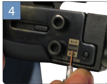
4 Ensure cable preparation is correct. Use gauge on VT tool to check the center conductor length.
