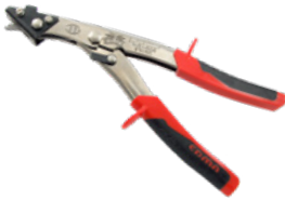
SUPER SNIP SHEAR Part #X HC1451 Cuts specialty corners or notches in straight run molding and to cut straight run length.
