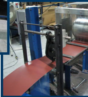
This machine creates custom-formed accessories that include corners, tee fittings and outlet boxes.
