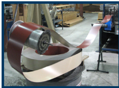
Belden utilizes a roll form machine to produce exact sizes of cable molding.
