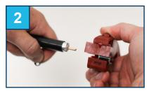
Rotate the tool around the cable to cut through the jacket, braid and dielectric. Pinch the tool on top of the cable and spin an additional tum, then pull the tool off axially to remove the cut jacket, braid and dielectric.
