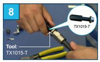
Use an insertion tool to aid in the installation. Continue to push and rotate the tool until the connector is fully installed.
