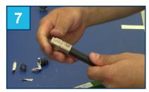
Guide the cable into the back nut and ensure it's properly seated before applying force.
