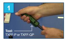
Insert the cable into the first cut side of the coring tool and rotate the tool several times until you hit the stop in the tool.
