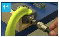
Guide the center conductor of your prepped connector into the front body and insert until it clicks together.
