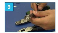
Proper installation is when you can visually ensure the dielectric is flush with the end of the connector.
