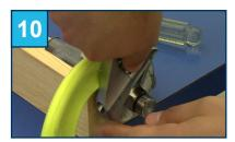
Insert the front body of the connector into the equipment. Hand tighten, and use an adjustable wrench to tighten another 1/8 to 1/4 turn.
