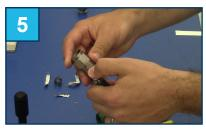
Use the second mark on the connector to measure your center conductor length.
