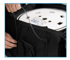
Secure the fiber in the rubber cable slot and thread the fiber cable through the two cable loops
