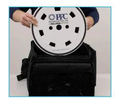
Insert the fiber reel so the tabs on the bottom of the bag fit into the notches on the reel
