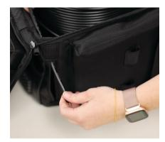
Feed the cable end through the open side of the bag and through the storage loop and close the bag.
