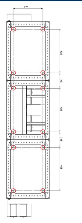
Left: Schematic view showing the positions of the floor fixing holes (circled in red).
