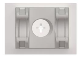
■ On occasions when the grooves in the Miniflex Distribution Cable cannot be satisfactorily aligned with the retention features in the cable clips, it is possible to adjust the clip position 1-2mm by loosening the screw, relocating and then retightening the screw.
