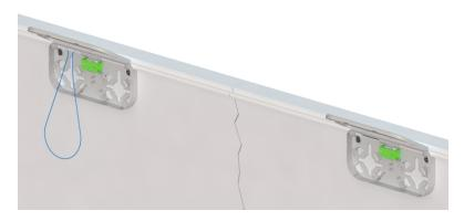
■ Following the direction of the main distribution point, cut the 900µm subscriber fiber at the next available point of entry.
