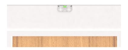
■ The Fiber Entry Box is mounted over the Miniflex Distribution Cable at the point of entry transition between corridor and dwelling. This is typically above or close to the door.
