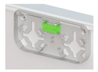
■ Reposition the Fiber Entry Box over the window cut and mark the position of the two mounting holes. Use a spirit level if necessary to ensure that the box is level.
