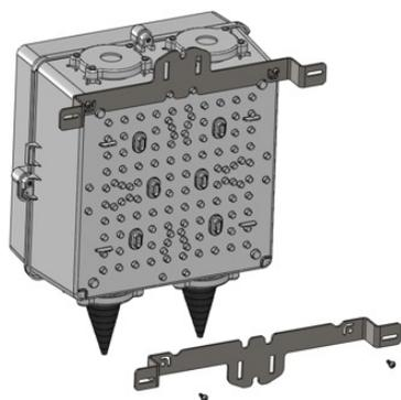
1. Before mounting, attach the brackets with the four provided screws.
