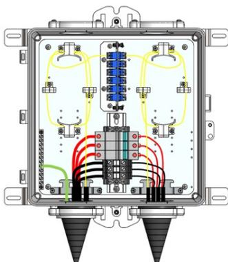
1. Connect any ground or tracer wire to the ground block on the left side.
