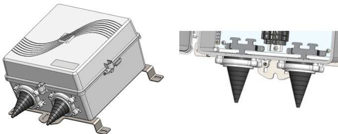
1. Two Rubber cone grommets are provided. – Use one for incoming cables and ground wire, and the second for outgoing cables.
