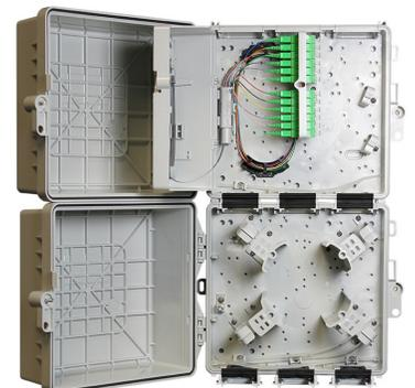
**PAT — Pedestal Access Terminal** offers a flexible solution for FTTH deployments. Designed to fit in pedestals as small as six inches (nominal diameter), these enclosures can be deployed in both greenfield and brownfield projects. Equipped with up to 12 SC/APC adapters, a splice tray, or both. The terminals make the task of distributing individual drop cables easy.
