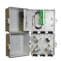
**PAT** — **Pedestal Access Terminal** offers a flexible solution for FTTH deployments. Designed to fit in pedestals as small as six inches (nominal diameter), these enclosures can be deployed in both greenfield and brownfield projects. Equipped with up to 12 SC/APC adapters, a splice tray, or both. The terminals make the task of distributing individual drop cables easy.
