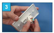
Align the two small latches on the bottom of the accessory (circled in blue above) with the corresponding lip on the wall plate, and confirm the wall plate lip holds the accessory properly in place.
