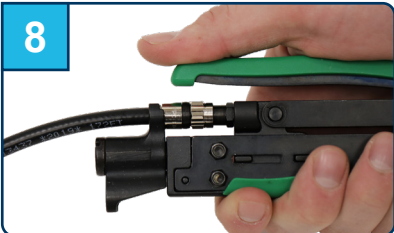
Properly seat the connector in the VT tool and fully compress it.
