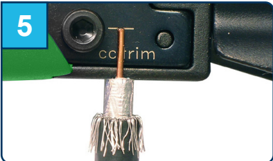
Use the gauge on the VT tool to check the dimension of the center conductor.
