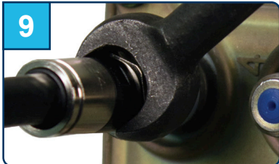
Install the connector onto the port and tighten to recommended torque.
