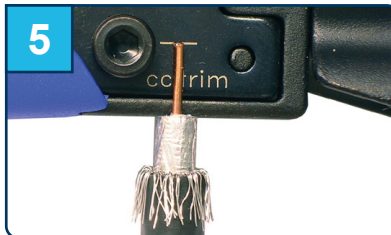
5 Use the gauge on the VT tool to check the dimension of the center conductor.
