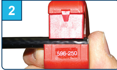
2 Using a fixed blade with a prep tool in good condition, prepare the cable to 5/16" x 1/4" x 1/4" dimensions. Use the edge of the tool if there is no stop.
