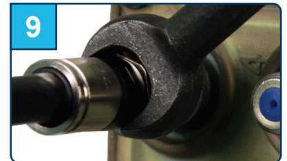
9 Install the connector onto the port and tighten to recommended torque.
