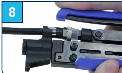
8 Properly seat the connector in the VT tool and fully compress it.
