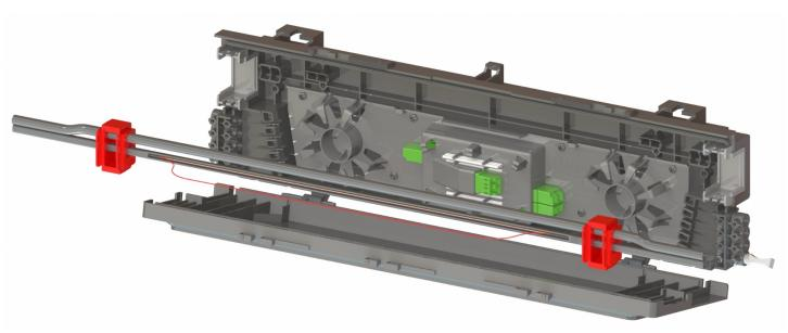
**Step 4:** Fit the closure over the distribution cable and securely seat the cable grommets into the closure port locations.
