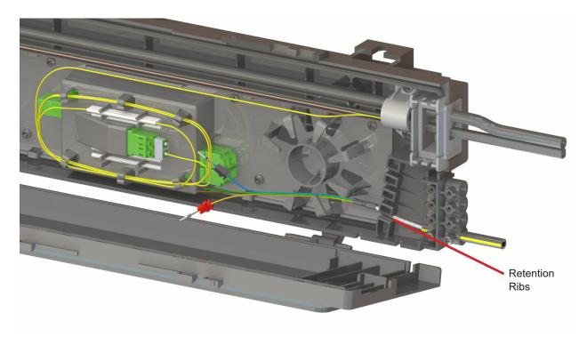
Step 4: Re-tighten the two M2.9 x 8 screws to secure the ADSS outer jacket into the drop cable port.
