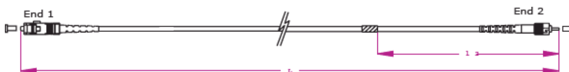
Fig.1: Simplex patchcord schematic
